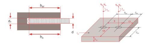
$h_{min}$  = Min. concrete thickness (mm)
